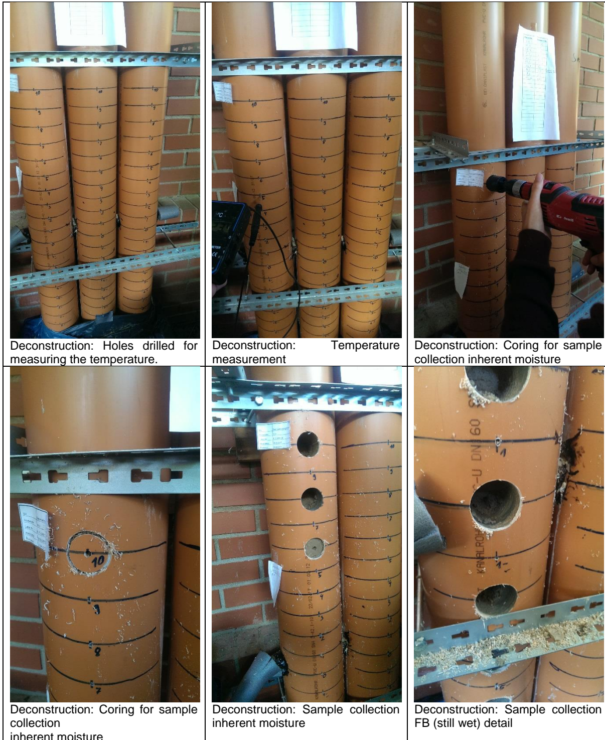
Figure 20: Deconstruction photo documentation (14 June 2017)
