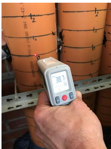
Figure 11: Measuring principle surface temperature on the sewage pipes
