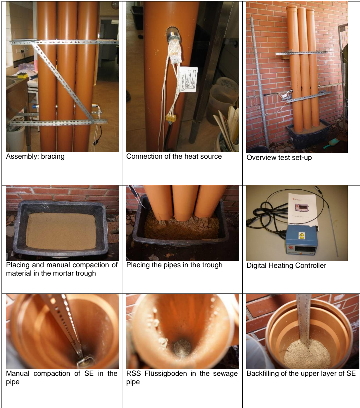
Figure 2: Photo documentation of the test set-up
