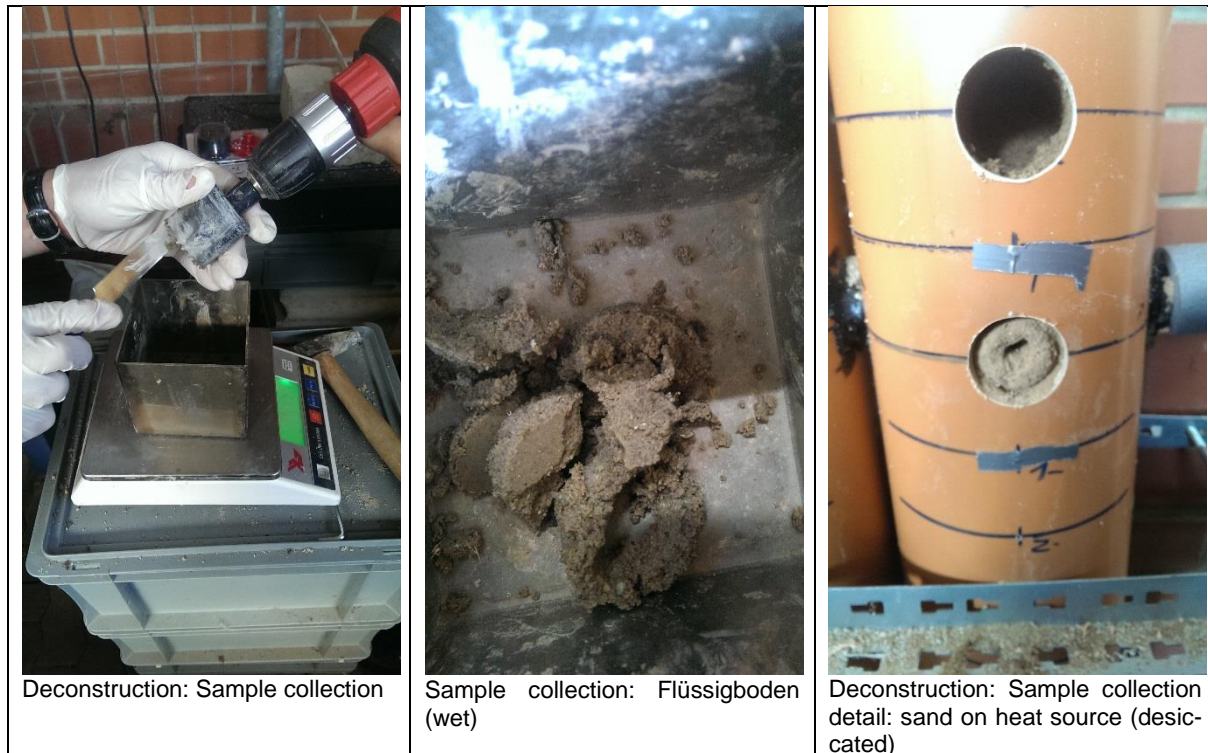
Figure 21: Deconstruction photo documentation (14 June 2017)
