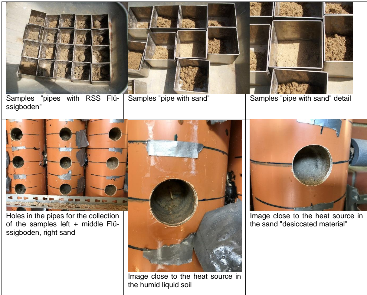
Figure 22: Deconstruction 14 June 2017 photo documentation optical desiccation sand/moist condition Flüssigboden
