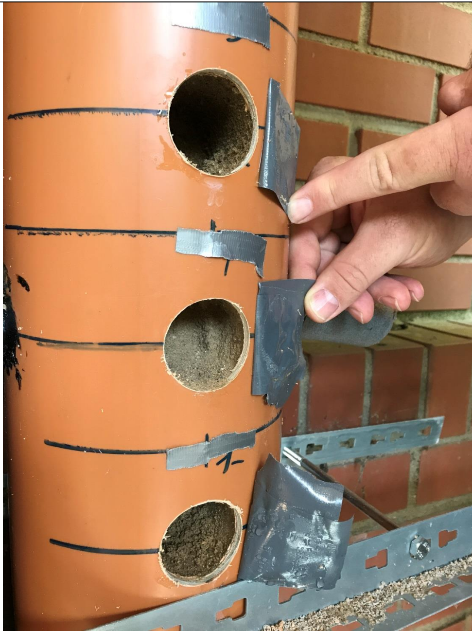
Deconstruction: 19 June 2017, sand in position 0 – dry and in positions -1 and +1 wet
