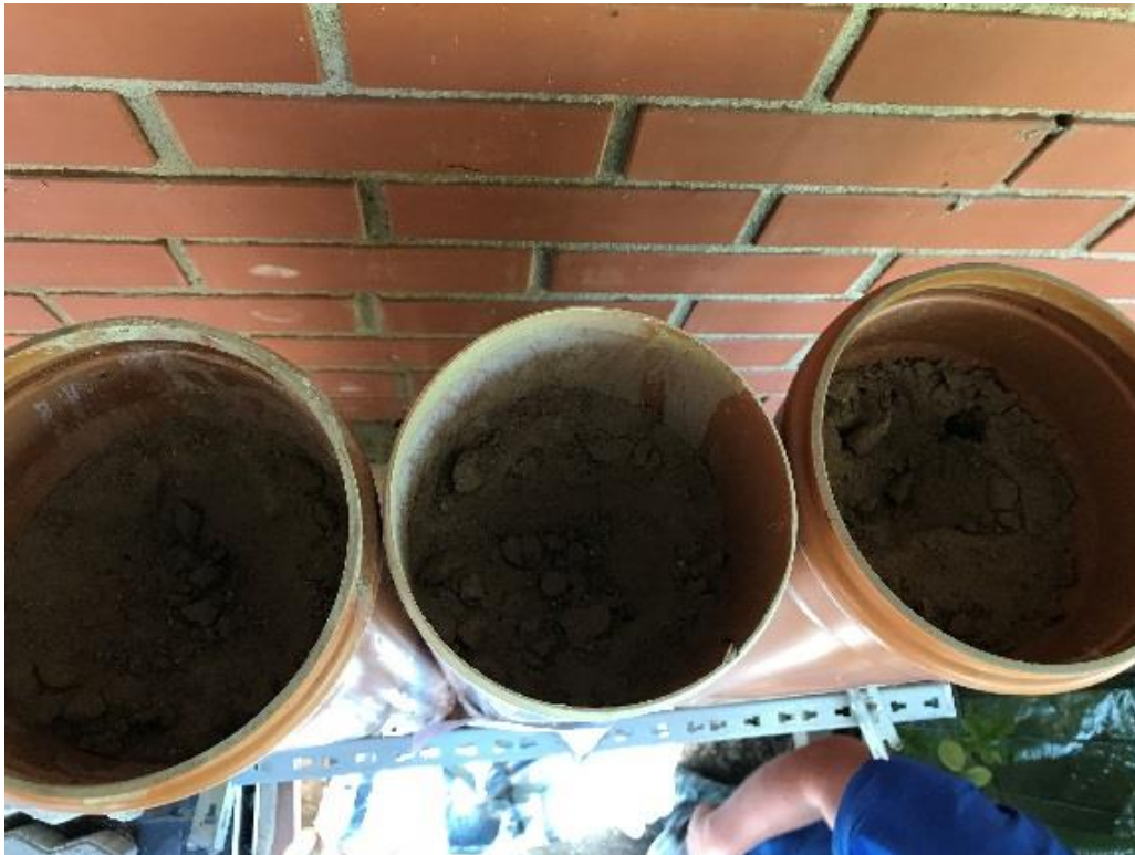
Figure 19: Top view on the test set-up (determination of inherent moisture in covering sand over Flüssigboden/sand)
